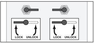
Figure 4. Configuration to extend the table beyond the regular stopping position.
